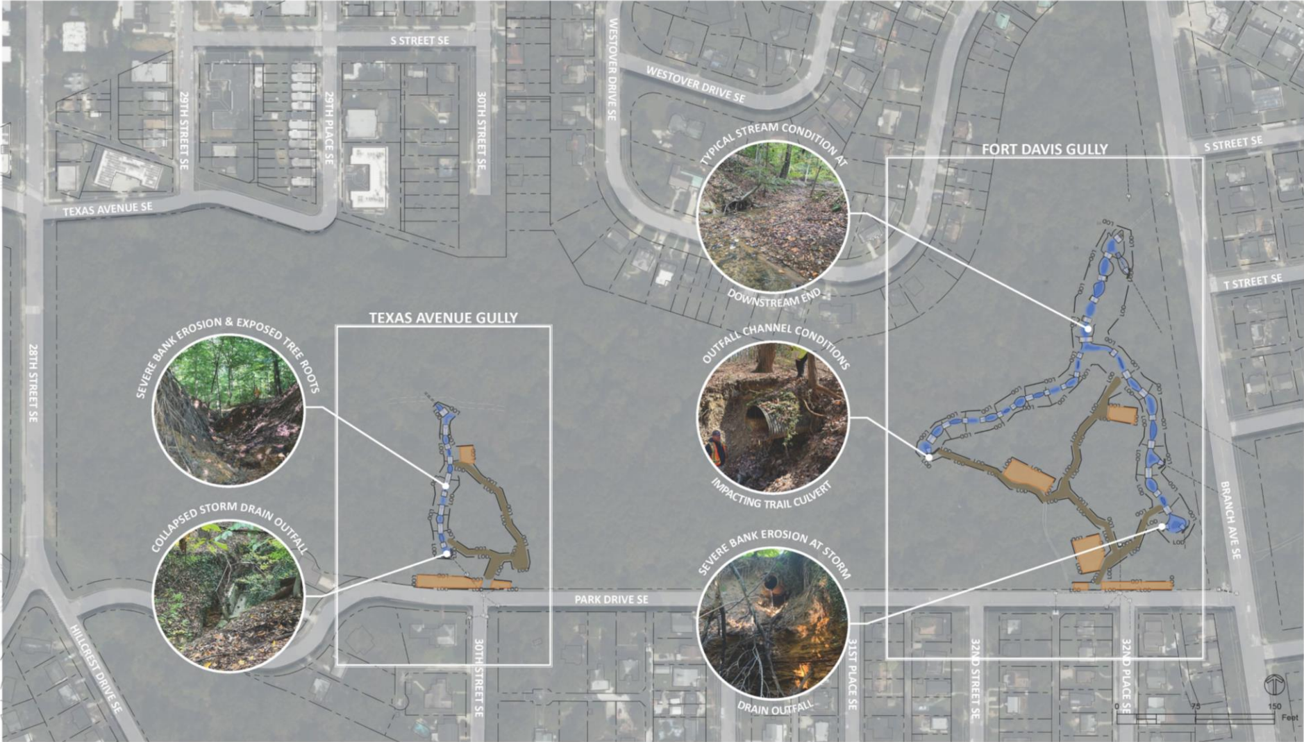
PARK DRIVE GULLY OUTFALL AND STREAM RESTORATION TEXAS AVE & FORT DAVIS GULLY - PROPOSED CONDITION VICINITY PLAN WASHINGTON, DC
